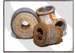
Corrosion products Rust / Calcium carbonate
